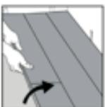
Separate the whole row by lifting it up delicately at an angle. To separate the planks, simply lift each plank vertically to disengage the end joint.
